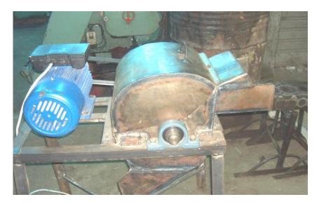
Fig. 1. The developed chopping machine.
