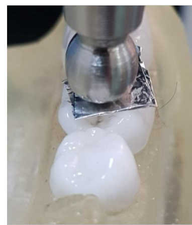
Figure 1: Tin foil sheet placed between the loading applicator and the
