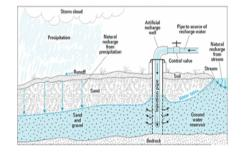
Fig. 2 Artificial recharge of groundwater aquifers [30].
