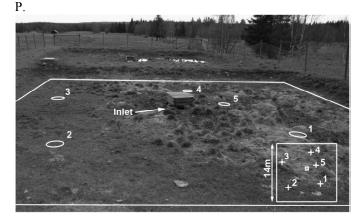
**Fig. 7** Illustration of filter the bed and locations of sampling [44].
