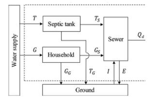
**Fig. 5** System boundary and component reproduced from Watanabe et al. [39].
