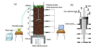
**Fig. 6** Schematic diagram for a) the simulator of the SWIS, b) the sampler of the gas [41]
