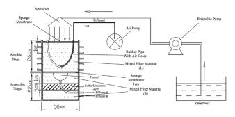
**Fig. 4** A schematic diagram of the lab-scale SISSAD reactor [37].
