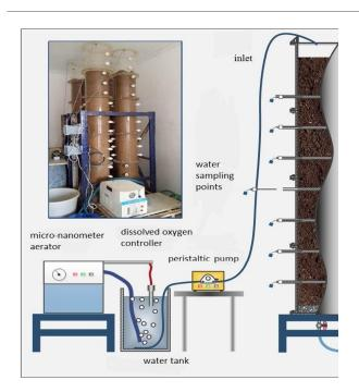
Fig. 3 Soil column setup supplied by fine bubbles aeration technology [1].
