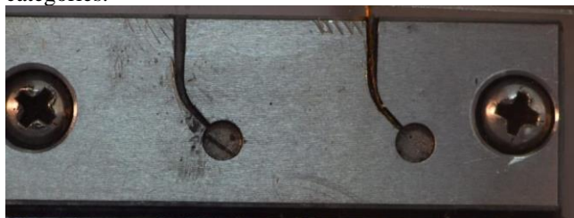
Figure 2. File within the simulating canal inside the stainless steel template, overlaid by glass film.
