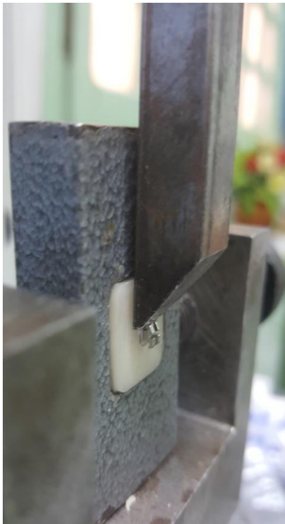
Figure 1: specimen fixed to universal testing machine
