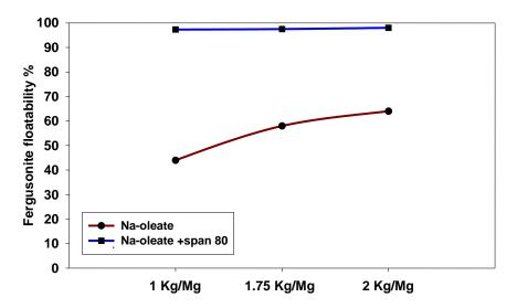
Fig. 4: Effect of collector dosage on floatability of fergusonite using sodium oleate and mixture of sodium oleate and span 80.
