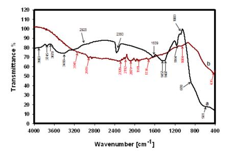
Fig. 9: FT-IR spectra of fergusonite (a), fergusonite treated with mixed collector (b).
