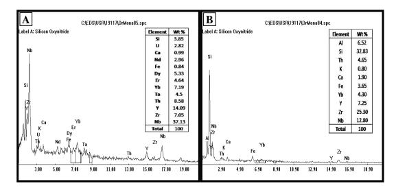
Fig. 10: EDX analysis data of froth (A), sink (B) products.
