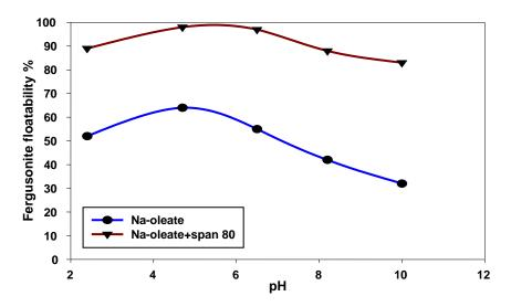
Fig. 5: Effect of pH on floatability of fergusonite surface using Na-oleate and the mixture collectors.
