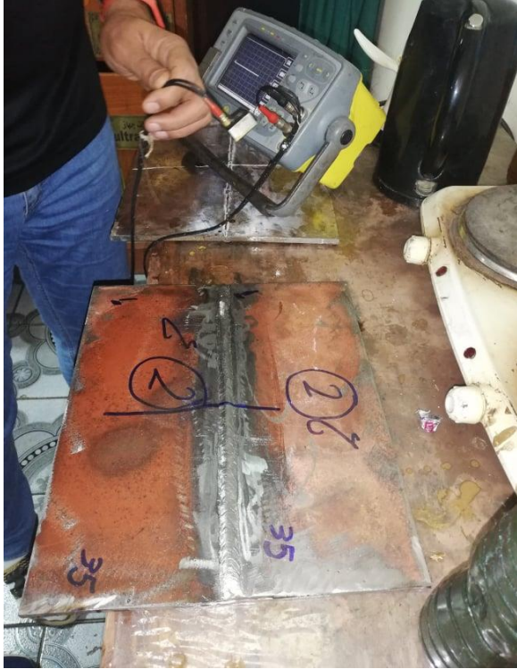
Figure 12: Ultrasonic Test (UT) for accepted welding joint
