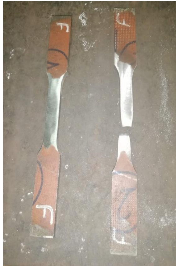
Figure 17: Welding joint after tensile test
