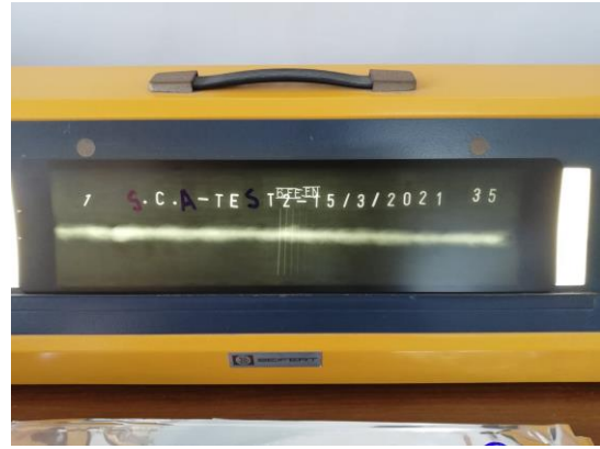
Figure 13: X-ray test for accepted welding joint
