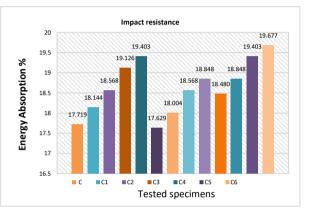
Figure 10: Effect of waste rubber on energy absorption.
