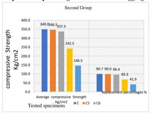
Figure 7: Average compression strength at different replacement percentages of rubber as both coarse and fine aggregates.
