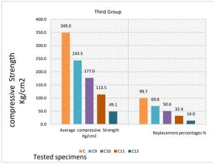
Figure 6: Compression strength at different replacement percentages of rubber as fine aggregates.
