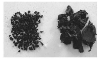
Figure 1: Grinded rubber and shredded rubber
