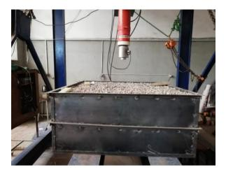
Figure 3: The steel container filled with subbase layers.
