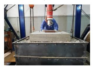
Figure 2: The specimen was placed in the middle of container and the steel plate was placed in its center.
