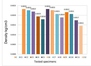
Figure 9: Effect of rubber waste percentages on density
