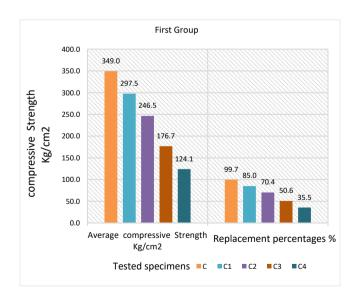
Figure 5: Compression strength at different replacement percentages of rubber as coarse aggregate.
