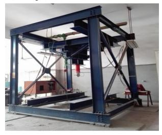
Figure 1: rigid steel frame supported on the laboratory rigid floor
