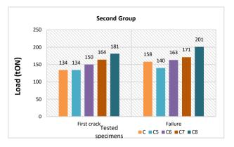
Figure 12: Loading test for second group samples.
