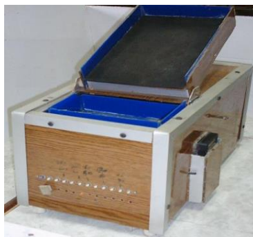
Figure (3): Digital device used for measuring the friction angle.
