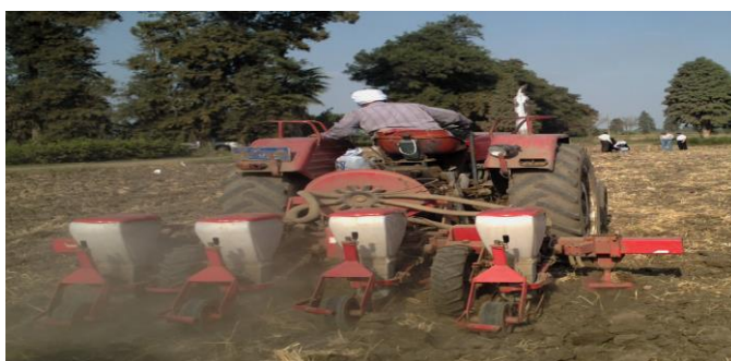
Fig. (1) Modified pneumatic Nibex planter while working in the field.
