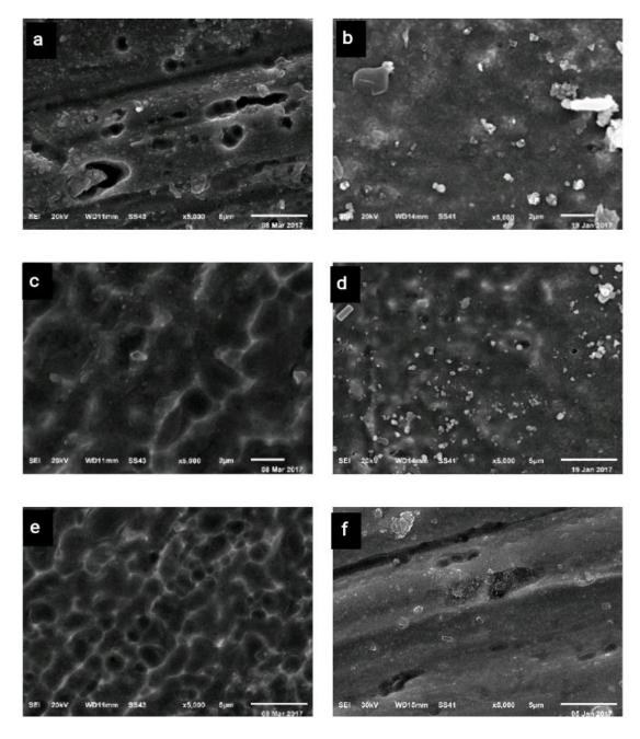
Fig.2: SEM images of Cu NiTi specimens after immersion in the testing solutions. a- Control
