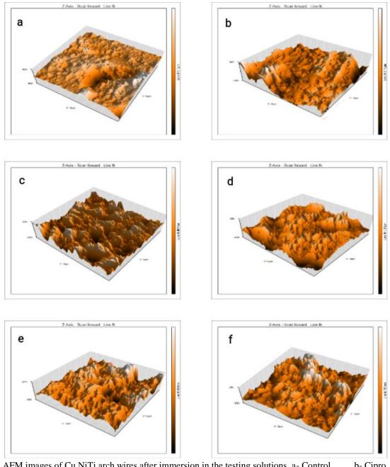
Fig. 1: AFM images of Cu NiTi arch wires after immersion in the testing solutions. a- Control
