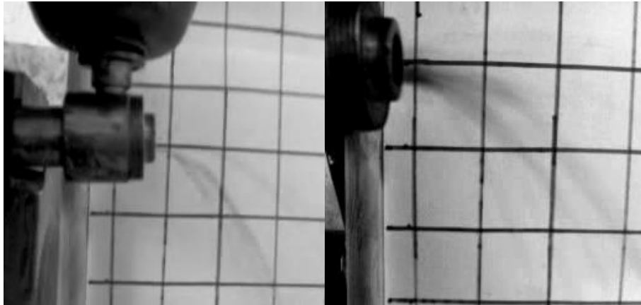
Fig. (6): The inclination curve of seed out for metering device after deletion the rotor unit
