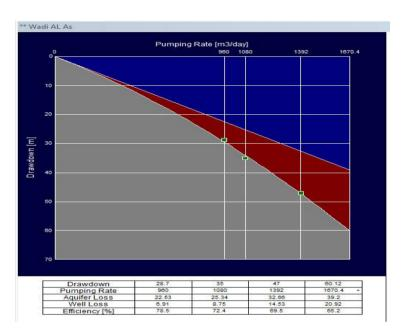
Figure 10 Analysis of Step-Drawdown Test Data of the Well: Al-Assuity.
