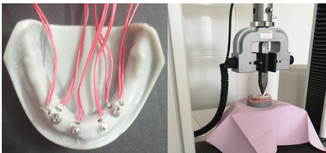
Figure 5: Stain gauge installation and stress analysis using the universal testing machine.
