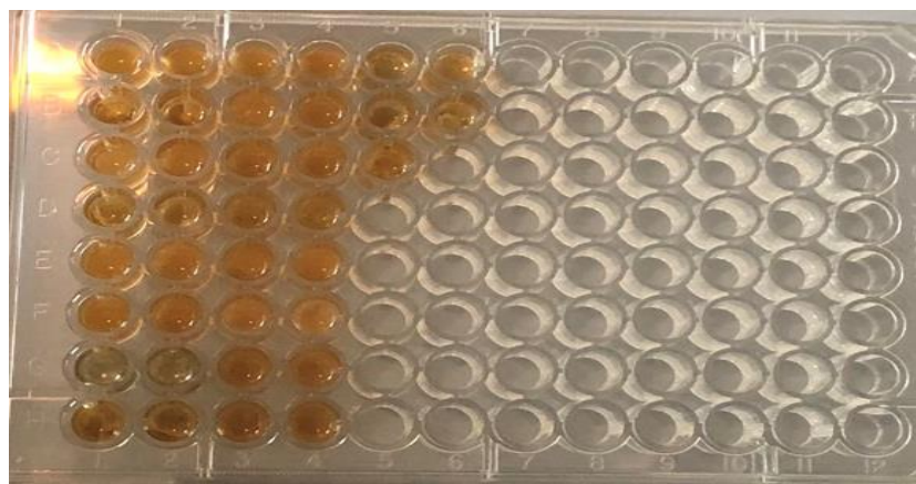
Fig. 7: Microtiter plate before crystal violet staining.
