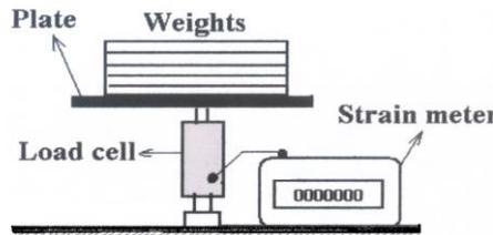
**Fig. (9): Calibration set-up for the load cell.**
