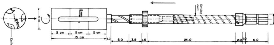
**Fig. (8): The soil samples collector.**
