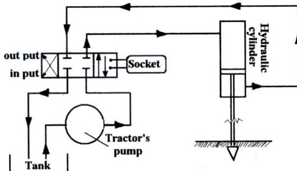
Fig. (7): The hydraulic system connections
