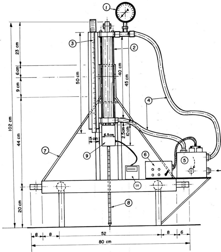
Fig. (3): Schematic diagram of the developed device showing arrangement to collect soil cone index data.
