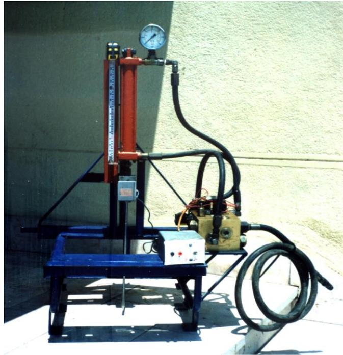
Fig. (4): Photo of the developed device showing arrangement to collect soil cone index data.
