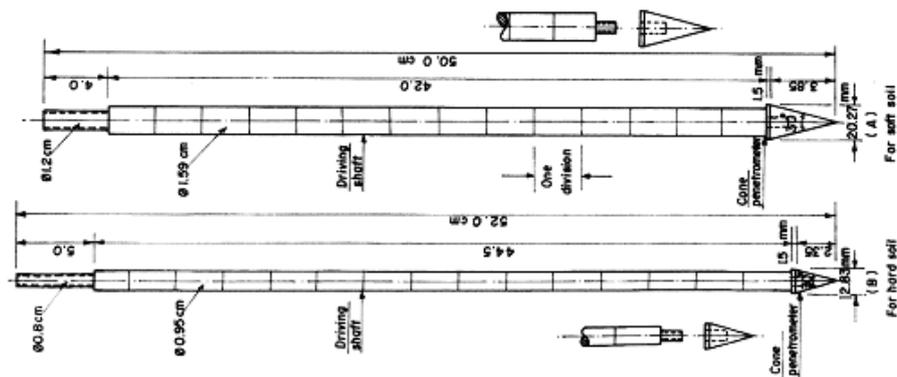
Fig. (5): Details of the used steel shafts with its end cone tip used in the developed penetrometer.
