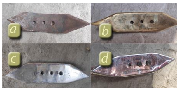
Fig. 1. Four type of chisel plow shares (a: iron, b: copper, c: aluminum and d: stainless steel)
