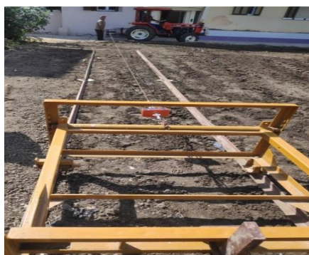
Fig. 2. Open air soilbin with a digital electronic dynamometer
