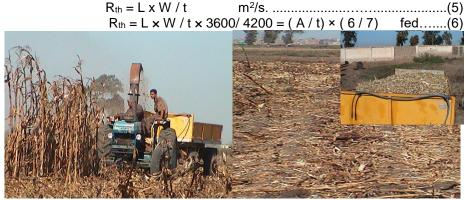
Fig. (3) Double chopper machine during and after cutting corn stalk
