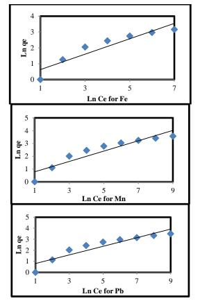
Fig. 8: Freundlich isotherm model for Fe Mn and Pb metal adsorption on SCB.
