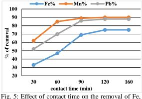
Fig. 5: Effect of contact time on the removal of Fe, Mn and Pb using SCB adsorbent.
