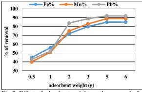
Fig.3: Effect of adsorbent weight on the removal of Fe,Mn and Pb using SCB adsorbent.
