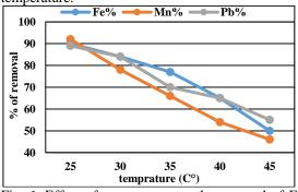
Fig. 6: Effect of temperature on the removal of Fe, Mn and Pb using SCB adsorbent.
