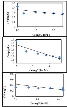
Fig. 7: Langmuir isotherm model for Fe, Mn and Pb metal adsorption on SCB.
