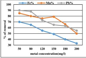
Fig.4: Effect of initial metal concentration on the removal of Fe,Mn and Pb using SCB adsorbent.
