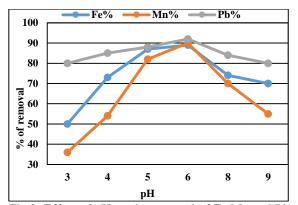
Fig.2: Effect of pH on the removal of Fe,Mn and Pb using SCB adsorbent.
