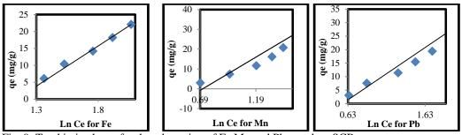
Fig. 9: Temkin isotherm for the adsorption of Fe Mn and Pb metal on SCB.
