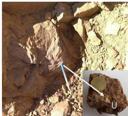
Fig. 3. Mineralized mylonitic normal N15°W shear zone dipping 86° to SW in Abu Harba granites with visible oval secondary uranium mineral, top view, G. Abu Harba area.
