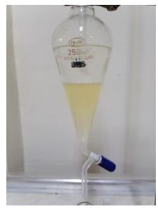
Fig. 1. Separation of the organic layer using a separating funnel
