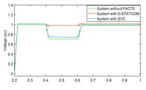
Fig. 7. Double line - ground voltage magnitude with and without D-FACTS.
