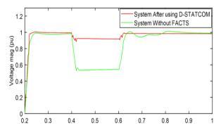
Fig.8. Three phase - ground voltage magnitude with and without D-STATCOM.
