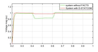
Fig. 6. Single-line to ground voltage magnitude with and without D-STATCOM.
