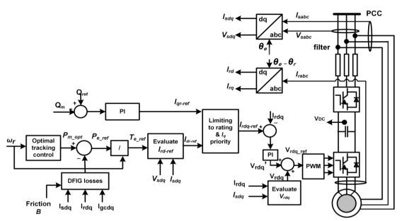
Fig.4. Control scheme of rotor side converter.
