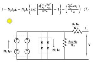
Fig.5. The equivalent circuit of PV array.
