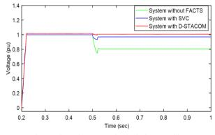
Fig. 9. The voltage magnitude during a sudden heavy load with and without D-FACTS.
