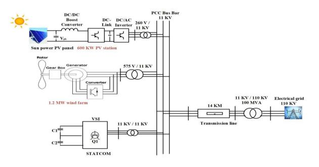
Fig.3. proposed Grid with PV/wind hybrid power system and D-STATCOM.
