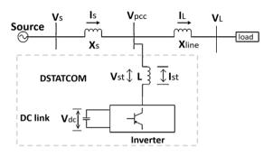
Fig.2. D-STATCOM with the electrical power system.
