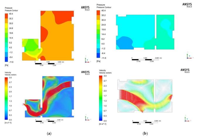
Fig.9. (a) Zad El-Mosafer studied room plan that Clarifies Pressure Contours (Pascal is the SI unit for pressure equal to (40.4 PA) & Velocity Vectors (wind velocity equal to 3 m/sec; (b) kom El-Dikka studied room plan.
