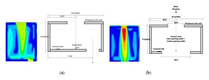
Fig.6. (a) Stagnation condition inside cross-ventilation single rooms;(b) Venturi condition inside cross ventilation single room & the Simulation results examples with their velocity [50].
