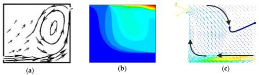
Fig.5. (a) Sketch generated by the observation of the phenomenon of natural ventilation of buildings [30]; (b) Illustrates the Contours of temperature [30]; (c) Velocity vectors with note of curves showing the main flow field [30].
