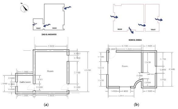
Fig.8. Zad El-Mosafer studied room plan that shows wind direction coordination & detailed room dimensions; (b) kom El-Dikka studied room plan that shows wind direction coordination & detailed room dimensions.
