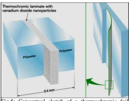
Fig.5: Conceptual sketch of a thermochromic foil incorporating a laminate with VO2-based nanoparticles between two foils of (polyester, PET) <sup>(1)</sup>
