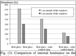
working plane in the reference room with different window glazing <sup>(11)</sup>
