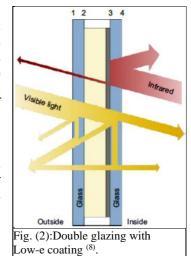
reflected or absorbed and emissivity reduced <sup>(8)</sup>. By coating at least one of the four glass surfaces of a double-glazing unit with a layer of material highly reflective to IR radiation (low-E), it is possible to obtain insulating glazing with high thermal performance. Instead of radiating part of
