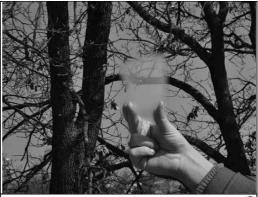
Fig.(6) View through a monolithic aerogel sample <sup>(5)</sup>
