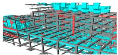
Fig. 15-3D model for the hospital MEP system
