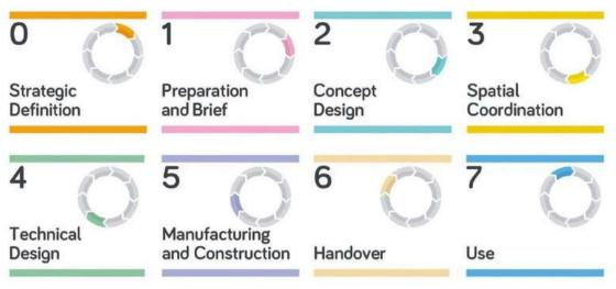
fig. 9 RIBA Plan of work (RIBA, 2020)
