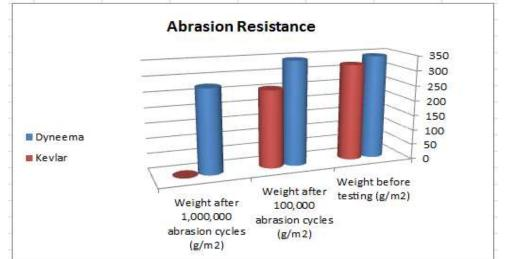
Figure 7. Weight before and after Abrasion Resistance Test
