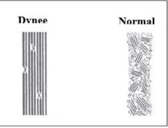
Figure 1. The difference between the molecular Chains arrangement of ordinary polyethylene (PE) and Dyneema (HPPE)<sup>[3]</sup>
