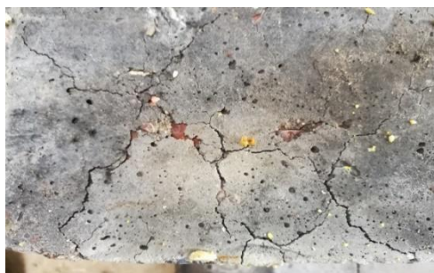
Figure (12) Hybrid mix specimen at 800 °C
