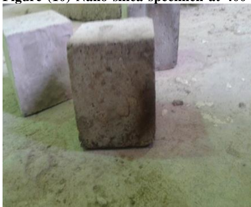
Figure (11) Nano clay specimen at 600 °C
