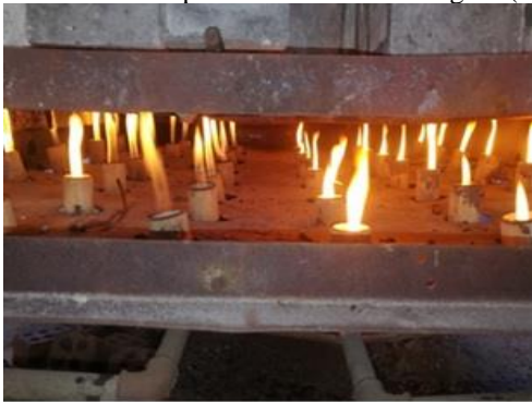
Figure (6) Burning of Concrete specimens
