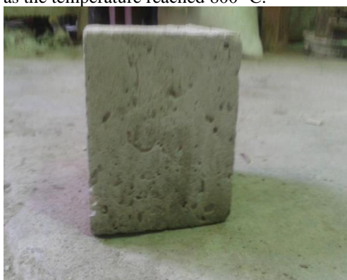
Figure (10) Nano silica specimen at 400 °C
