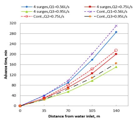
**Figure 5**: Advance time Vs distance from water inlet at different discharge rates with 5 surges and continuous flow irrigation
