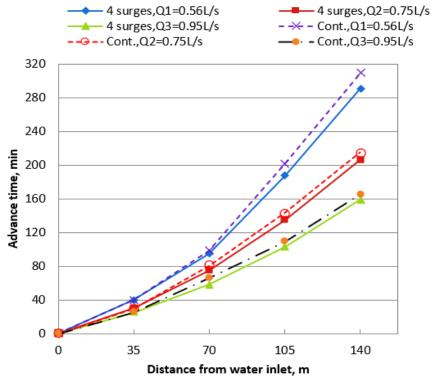
Figure 4: Advance time vs distance from water inlet at different discharge rates with 4 surges and continuous flow irrigation
