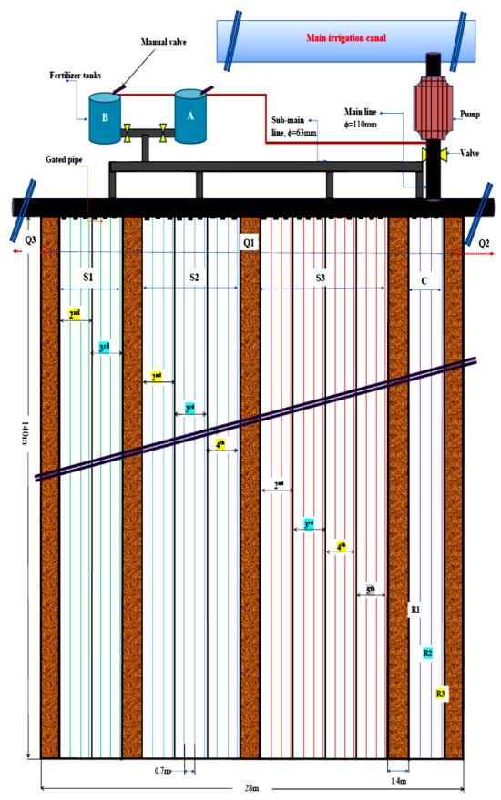
Figure 3: A schematic diagram of the experimental construction and design
