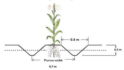
Figure 2: Geometry of furrow irrigation
