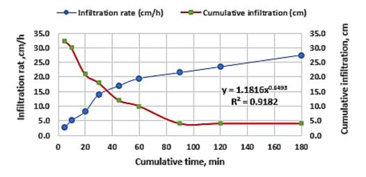
Figure 1: Cumulative infiltration and infiltration rate for soil of experimental site
