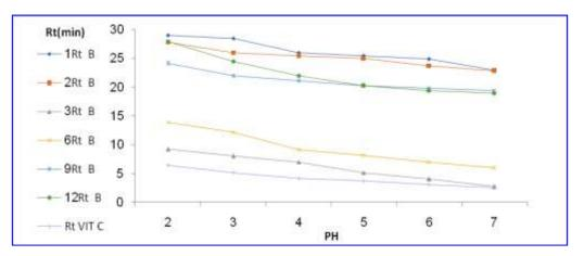
Fig 3: Effect of pH on retention time (RT) of soluble vitamins; B<sub>1</sub>, B<sub>2</sub>, B<sub>12</sub>, B<sub>9</sub>, B<sub>6</sub>, B<sub>3</sub> and vit. C.
