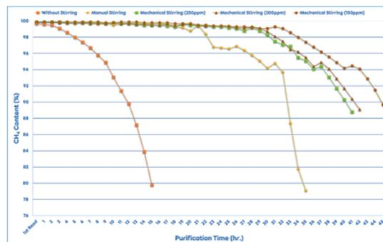
**Fig. 14. The effect of different stirring methods on methane content.**
