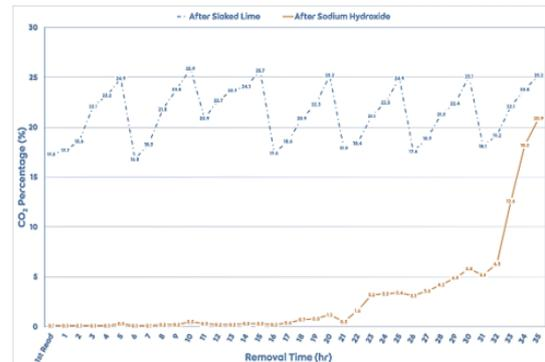
**Fig. 5. Carbon dioxide percentage in biogas after purification process using manual stirring method.**
