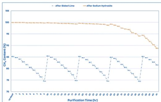
**Fig. 8. Methane content in biogas after the purification process using mechanical stirring method at speed of 250 rpm.**
