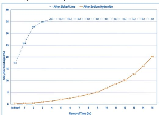
**Fig. 3. Carbon dioxide percentage in biogas after the purification process using non stirring method.**
