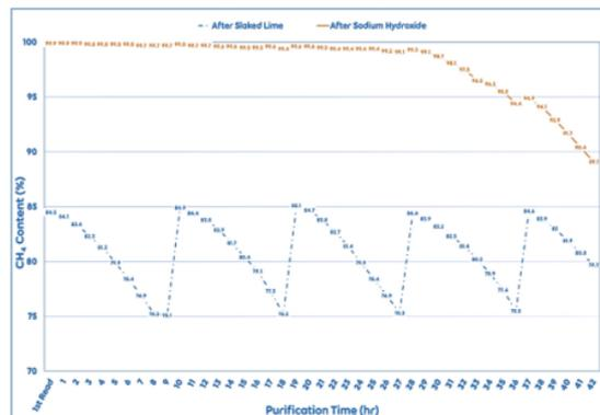
**Fig. 10. Methane content in biogas after the purification process using mechanical stirring method at speed of 200 rpm.**
