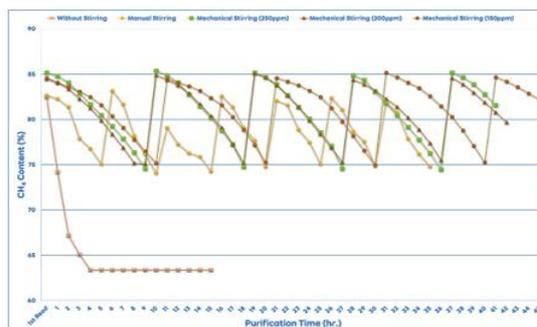
**Fig. 15. Comparison of methane content at slaked lime using different stirring methods.**
