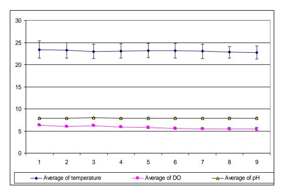
Figure (2): Average with standard error of Temperature (°C), pH values and Dissolved Oxygen (D.O.) in mg/l along Mahmoudia canal during the period from March 2008 to Jan. 2010.
