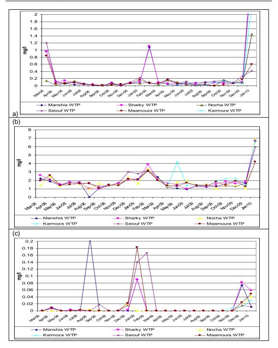
Figure (5): Average in mg/l of Free Ammonia (a), Nitrate (b) and Nitrite (c) for six AWCO WTPs effluent during the study period from March. 2008 to Jan. 2010
