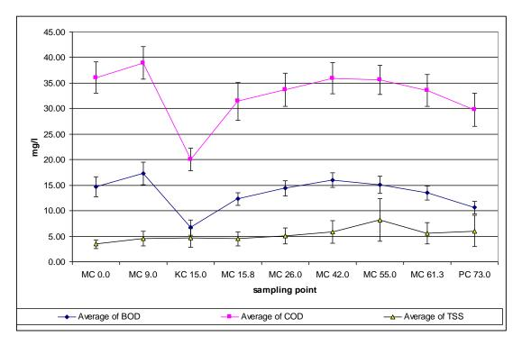
Figure (3): Average with standard error in mg/l of Biochemical Oxygen Demand (BOD<sub>5</sub>), Chemical Oxygen Demand (COD) and Total Suspended Solids (TSS) along Mahmoudia canal during the study period from March 2008 to Jan. 2010
