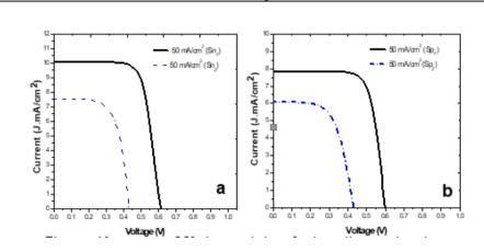
Figure(10): J-V characteristics of solar cell based on PSL prepared on (a): both sides (Sn<sub>4</sub> compared with that based one side (Sn<sub>2</sub>) and (b): both sides (Sp<sub>4</sub>) compared with that based on one side (Sp<sub>2</sub>).
