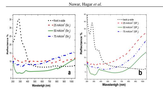
Figure(6): Reflectance of PSL samples prepared on (a): the front n-side (Sn<sub>1</sub>, Sn<sub>2</sub> and Sn<sub>3</sub>) and (b): back p-side (Sp<sub>1</sub>, Sp<sub>2</sub> and Sp<sub>3</sub>) corresponding to front n and back p-side without PSL layer.
