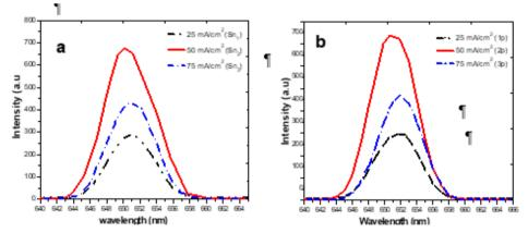
Figure(5): Photoluminescence of PSL samples prepared on (a): the front nside (Sn<sub>1</sub>, Sn<sub>2</sub> and Sn<sub>3</sub>) and (b): back p-side (Sp<sub>1</sub>, Sp<sub>2</sub> and Sp<sub>3</sub>)
