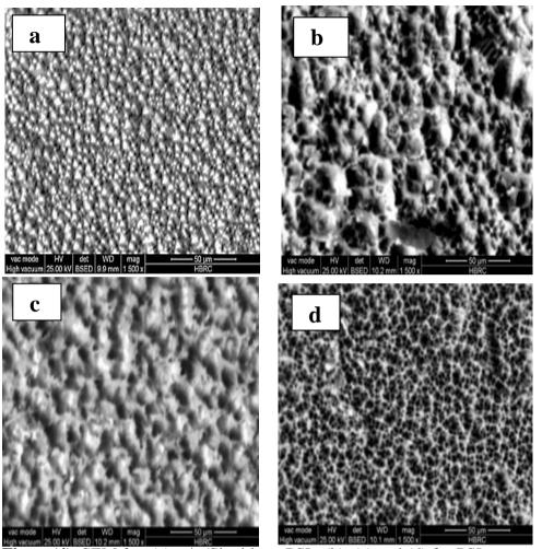
Figure(4): SEM for: (a): n<sup>+</sup>p/Si without PSL, (b), (c) and (d) for PSL
