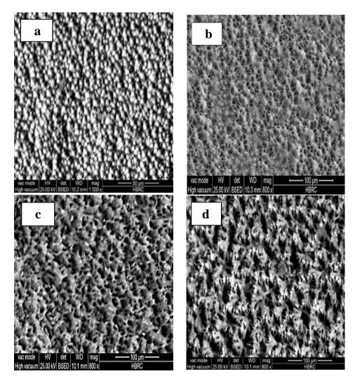
**Figure(3):** SEM of: (a) front n+p/Si without PSL, (b), (c) and (d) for PSL samples Sn1, Sn2 and Sn3 prepared at 25, 50 & 75 mA/cm<sup>2</sup> for fixed time of 25 min and electrolyte concentration (1:3)
