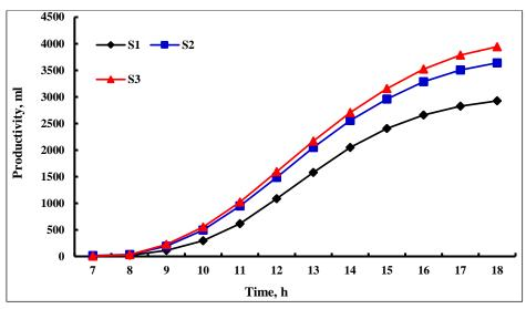
Fig. (7): Effect of PCM on the accumulated productivity of solar stills
