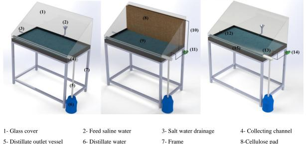
Fig. (2): Schematic diagram of experimental setup of solar stills
