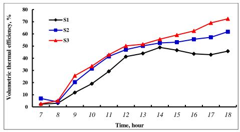
Fig. (8): Hourly average volumetric thermal efficiency versus time for the solar stills
