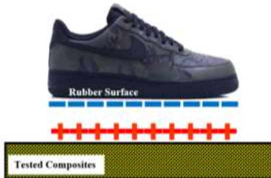
Fig. 6 ESC generated from the sliding of rubber sole on epoxy composites filled by rubber granulates of (2.0 – 3.0) mm size.
