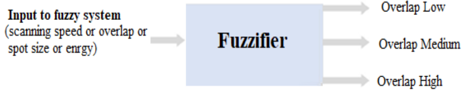
Fig. 7: Fuzzification of Fuzzy Systems Inputs
