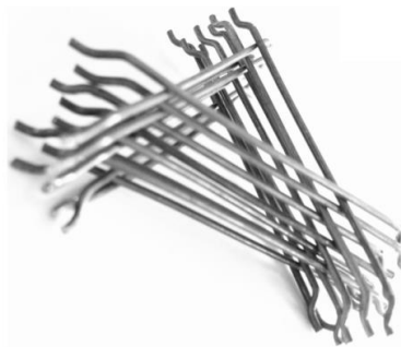
Fig. 5: Hooked steel fiber
