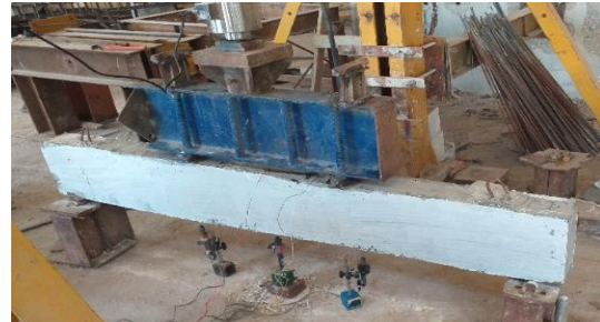
Fig. 7: Test set up and load pattern
