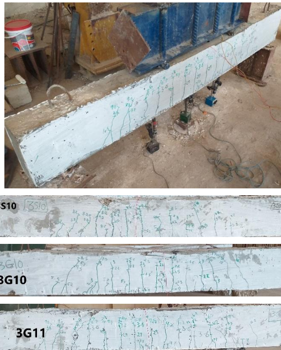
Fig. 12: Crack Pattern of beams at failure
