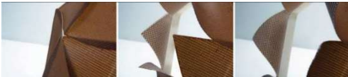
Figure 9: Humidity responsive 3D printed aperture. Low humidity: opened, High humidity: closed (Zuluaga et al., 2015).
