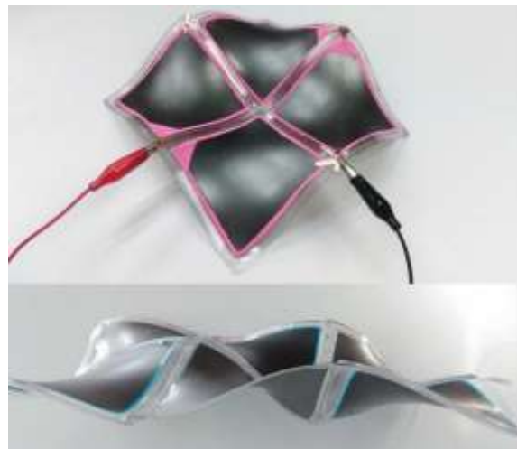
Figure 7: Dielectric shape shifting elastomer (Shimul, 2017).
