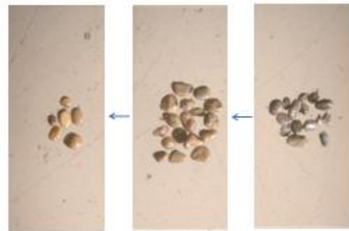
Figure (28): Photomicrograph showing the various stages for transformation of ilmenite to leucoxene due to leaching process, (X20)
