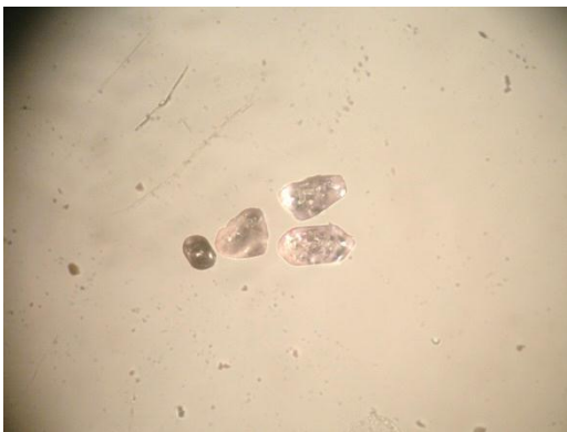
Fig.(31): Photomicrograph showing zircon grains of the separated sample from the gravimetric separation (grade A), (X20)
