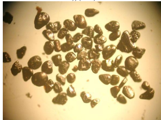
Fig.(33): Photomicrograph showing ilmenite grains of the separated sample from the gravimetric separation (grade B), (X20)
