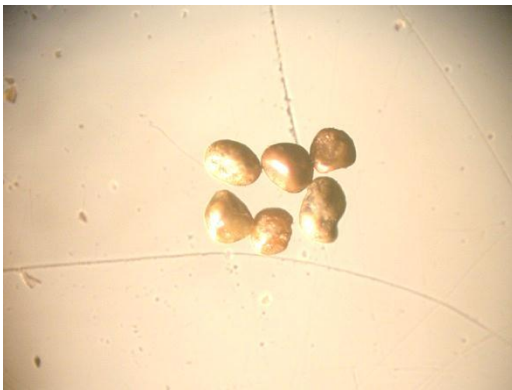
Figure (17): Photomicrograph showing leucoxene grains of the original rutile sample, (X20)
