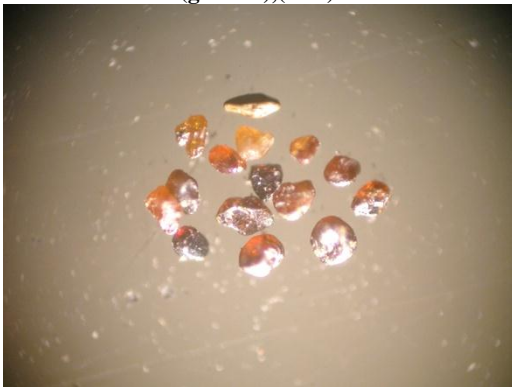
Fig.(30): Photomicrograph showing spheñ grains of the separated sample from the gravimetric separation (grade A), (X20)
