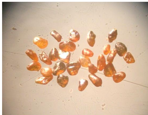
Figure (15): Photomicrograph showing sphen grains of the original rutile sample, (X20)
