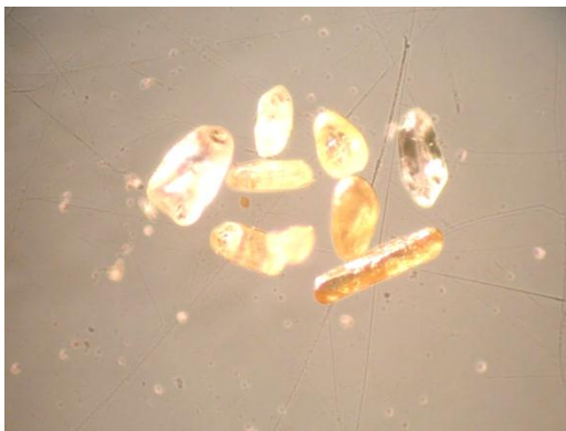
Figure (18): Photomicrograph showing zircon grains of the original rutile sample, (X20)
