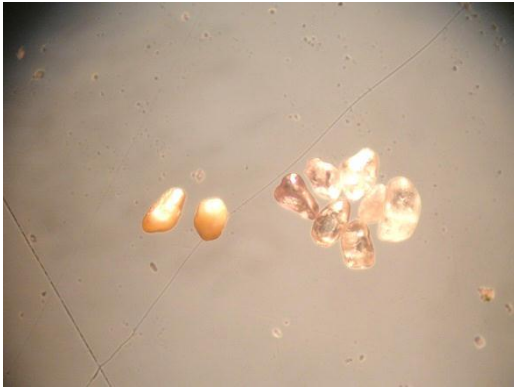
Fig.(35):Photomicrograph showing zircon grains of the separated sample from the gravimetric separation (grade B),(X20)
