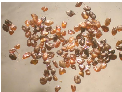
Figure (38):Photomicrograph showing sphen grains of the separated sample by magnetic separation, (X10)
