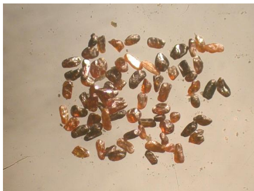
Figure (37):Photomicrograph showing rutile grains of the separated sample by magnetic separation, (X10)
