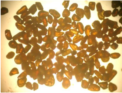
Fig.(29): Photomicrograph showing rutile grains of the separated sample from the gravimetric separation (grade A), (X20)
