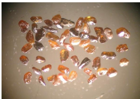
Figure (23): Photomicrograph showing rutile grains of the treatment sample by leaching process, (X20)
