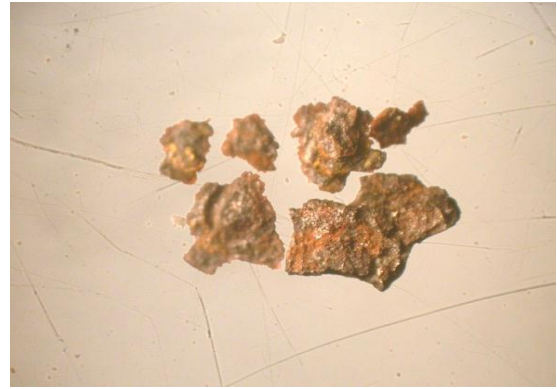
Figure (19): Photomicrograph showing secondary iron oxide grains of the original rutile sample, (X40)
