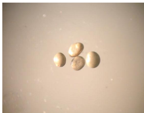
Fig(40):Photomicrograph showing leucoxene grains of the separated sample by magnetic separation, (X20)
