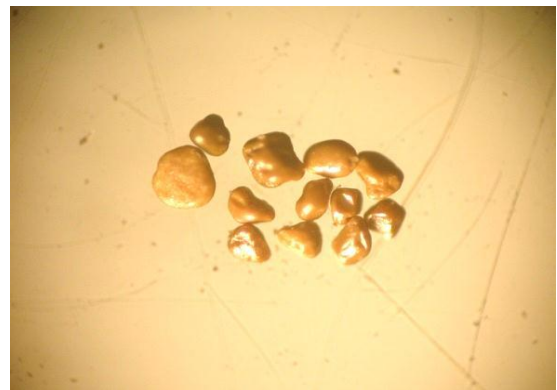
Fig.(21): Photomicrograph showing hematite grains of the original rutile sample, (X20)
