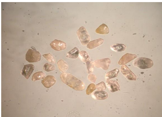
Figure (26): Photomicrograph showing zircon grains of the treatment sample by leaching process, (X20)
