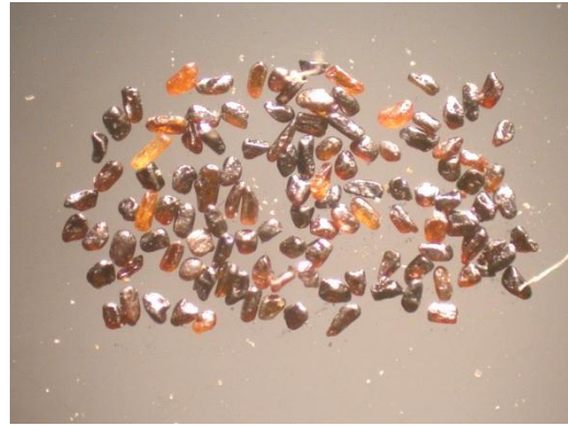
Fig.(32): Photomicrograph showing rutile grains of the separated sample from the gravimetric separation (grade B), (X10)
