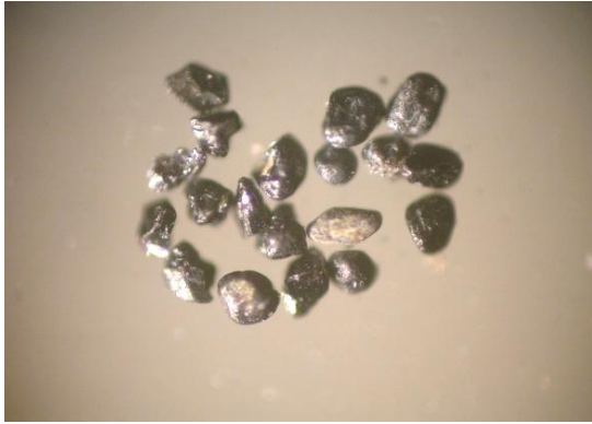
Figure (25): Photomicrograph showing ilmenite grains of the treatment sample by leaching process, (X20)
