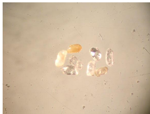
Figure (39):Photomicrograph showing zircon grains of the separated sample by magnetic separation, (X20)
