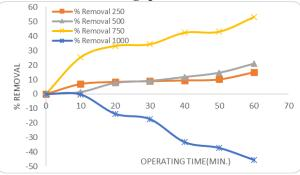
Figure (4): The Effect of Rotating Speed (rpm) on % Removal (C<sub>0</sub>=1000 ppm)
