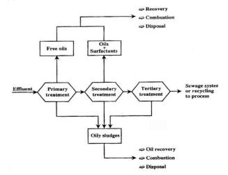
Figure (1): General Oily Wastewater Treatment
