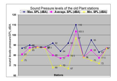
Fig. 4. Measured noise level in Dakhlia Sugar and Refining old plant
