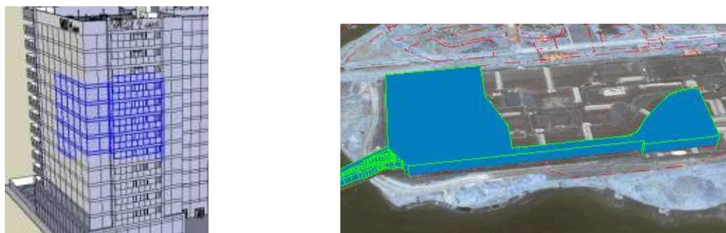
173 Fig 3. Studying the difference between 3D GIS and 3D Cadastre. 174 Left: Studying 2D, 2.5D, 3D physical shapes using 3D GIS. 175 Right: Studying closed volume of 3D space using 3D Cadastre as a 3D Geometric primitive. 176 Source: Ying, R. Guo, L. Li, and B. He, “Application of 3D GIS to 3D cadastre in urban environment”. in 3rd international workshop on 3D 177 cadastres: Developments and practices, 2012, pp. 25–26.
