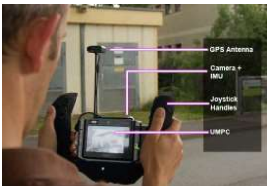
Fig 8. Using Vidente System to survey defined urban site, then converted the output data to an XML format in accurate geodatabase at ArcGIS software. Source: Researcher.
