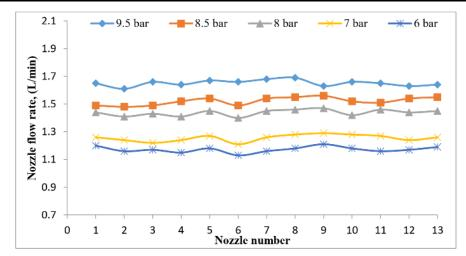
Figure 8. Distribution Uniformity of spraying machine for nozzle type (422HCC025).
