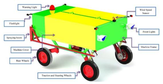
Figure 3. The isometric view of the spraying robot shows the main components with a non-spraying position.
