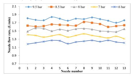
Figure 9. Distribution Uniformity of spraying machine for nozzle type (422HCC03).
