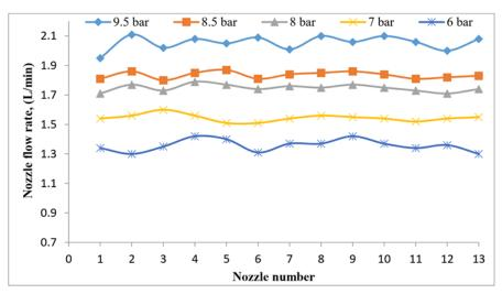
Figure 10. Distribution Uniformity of spraying machine for nozzle type (422HCC05).
