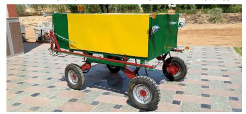
Figure 4. The spraying robot with a non-spraying position.
