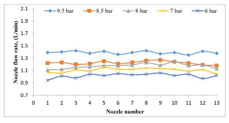
Figure 7. Distribution Uniformity of spraying machine for nozzle type (422HCC02).
