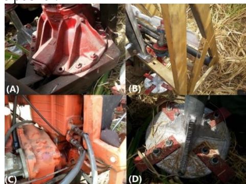
Figure 5. A. Gear box, B. Cutting system, C. Hydraulic system, D. Cutting disk.
