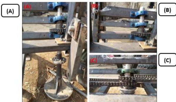
Figure 3. A. Height control Mechanism, B. Width control Mechanism, C. Transmission power for both cutting disks.
