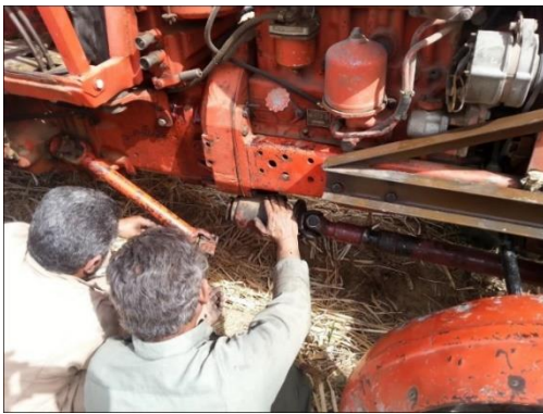
Figure 2. Power transmission shaft connection between machine and tractor.
