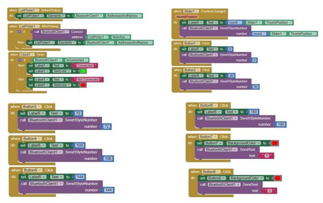
Figure 4. Programming code for the smartphone mobile app designed by MIT App Inventor.
