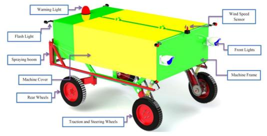
Figure 7. The main components of the spraying robot.
