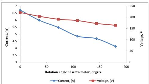
Figure 10. The relation between the voltage, current, and the servo motor rotation angle for one generator.
