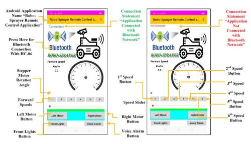
Figure 3. Smartphone mobile app designed by MIT App Inventor.
