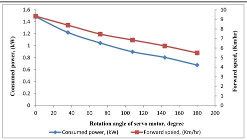
**Figure 9.** The relation between the forward speed, power consumed, and the servo motor rotation angle for one generator.
