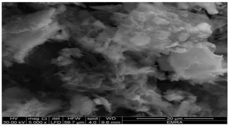
Figure 5. SEM Micrographs of Chabazite
