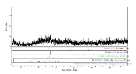
Fig. 2 Calcined kaolinite (meta-kaolinite)
