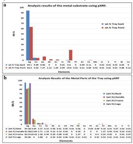
Figure (3) Shows pXRF analytical results of the metal substrate of <u>a</u>. the Indian Mughal tray, <u>b</u>. the Ottoman tray
