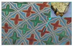
Figure (7) Shows digital microscope photomicrograph of the gilding layer beneath the enamel layer of the Ottoman tray.
