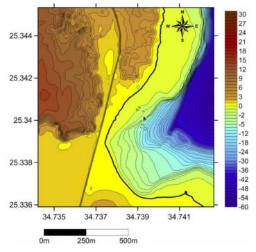
Fig. 2: Bathrymetric map of Marsa Abu Dabab showing gradient of depths.
