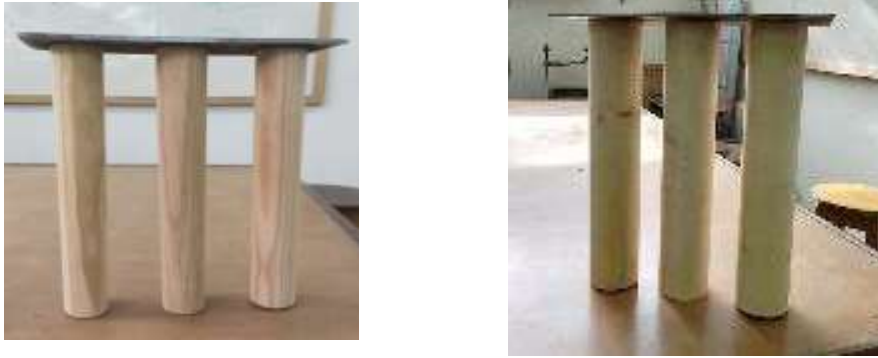
Fig. (3): Configuration of pile group, (a) : piles with D= 3 cm, (b) piles with D = 5 cm.
