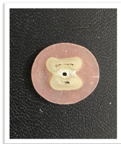
Figure 10: Push-out sample of MTA showing the cohesive failure.
