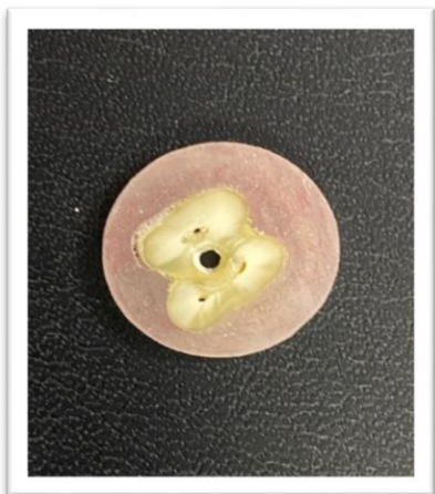
Figure 11: Push-out sample of Hydroxyapatite showing the adhesive Failure
